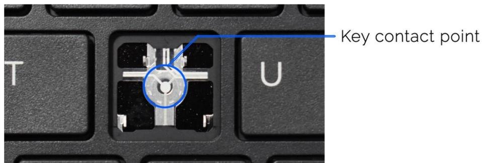
This will generally require no adhesive, as the key cap will hold the rubber cup in place when installed. If you wish to bond the new rubber cup to your keyboard, you can do so with a small amount of cyanoacrylate (also known as super glue or crazy glue - not included). Spread a *very thin* layer on the bottom surface of the rubber cup and set it into place. Allow it to dry **completely** before proceeding or you may risk damaging or inadvertently bonding other components!
