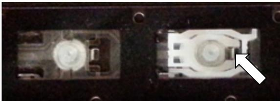
Hinges are pre-attached to each key for protection during shipping and must be removed to install. Take note of the orientation of the hinge mechanism to help you with placement.
