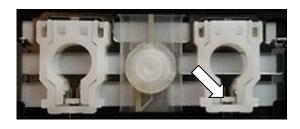
To install the hinge pieces, begin by hooking one end over the protruding metal tab located on the keyboard. A small flat screwdriver or blunt tweezers will assist you in this step.
