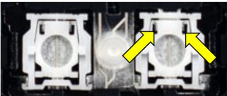
To install each hinge piece, begin by hooking one end over the protruding metal tabs located on the keyboard. A small flat screwdriver or blunt tweezers will assist you in this step. Keep the flattest side of the hinges facing up so it is able to properly receive the key cap.
