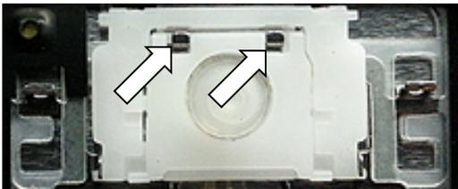
Hinges may be pre-attached to each key for protection during shipping and must be removed to install. Take note of the orientation of the hinge mechanism to help you with placement.
