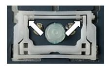
To install the hinge mechanism, begin by hooking one end over the protruding metal tabs located on the keyboard. A small flat screwdriver or blunt tweezers will assist you in this step.
