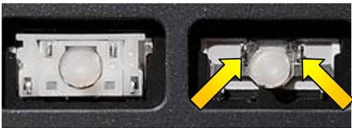
To install the hinge piece, begin by hooking one end over the protruding metal tabs located on the keyboard. A small flat screwdriver or blunt tweezers will assist you in this step. Keep the flattest side of the hinge facing up so it is able to properly receive the key cap.
