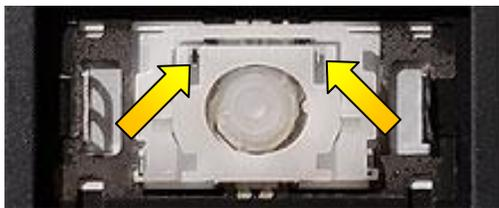
To install the hinge piece, begin by hooking one end over the protruding metal tabs located on the keyboard. A small flat screwdriver or blunt tweezers will assist you in this step. Keep the flattest side of the hinge facing up so it is able to properly receive the key cap.
