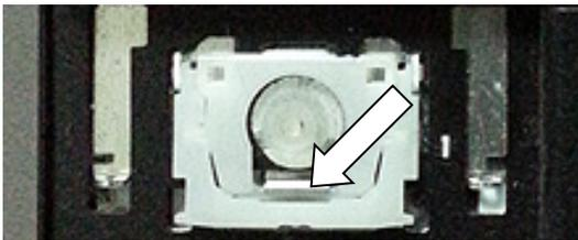
Hinges are pre-attached to each key for protection during shipping and must be removed to install. Take note of the orientation of the hinge mechanism to help you with placement.
